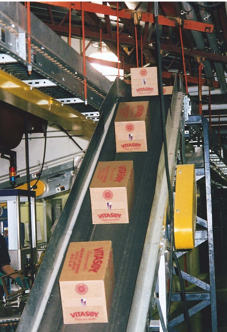
Filled cases of soy milk travel overhead from the capping and case-packing areas and descend on a conveyor toward the palletizing robot's picking station.
