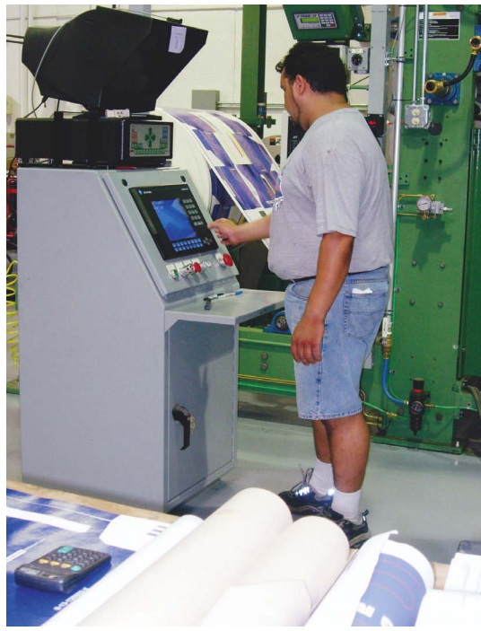
A press fingerprint, top, runs past the 68-in., two-lamp UV curing system. Press operator Oscar Ramirez, above, uses a video web-inspection system to check print quality on the new six-color CI-flexo press.
