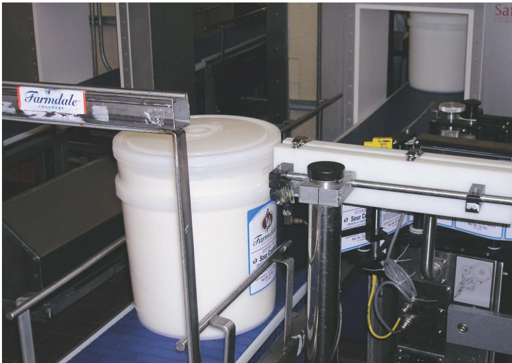
A new noncontact, ink-jet coder, left, applies the expiration date, batch number and time to the outside of an HDPE pail of sour cream. The inner workings of the ink-jet printhead, right, are revealed.
