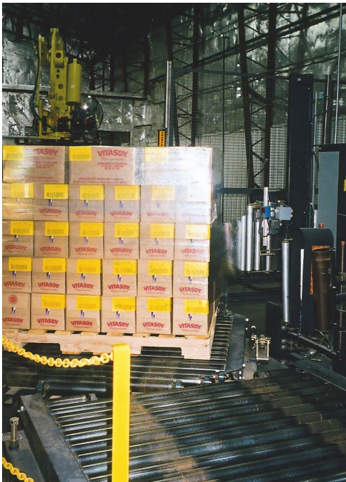
The turntable stretch wrapper finishes the load of soy milk cases, securing it in clear film. The robotic palletizer can handle more than 3 million lb/week.
