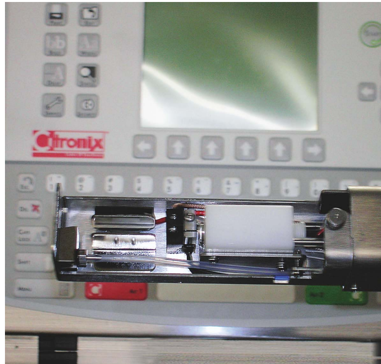
A new noncontact, ink-jet coder, left, applies the expiration date, batch number and time to the outside of an HDPE pail of sour cream. The inner workings of the ink-jet printhead, right, are revealed.
