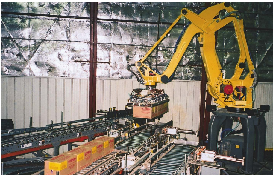
A robotic palletizing workstation added in 2005 occupies a minimum of space, but handles the maximum in payloads. Left, the robot's arm swings into action, grasping as many as seven cases and placing them on one of three pallets.
