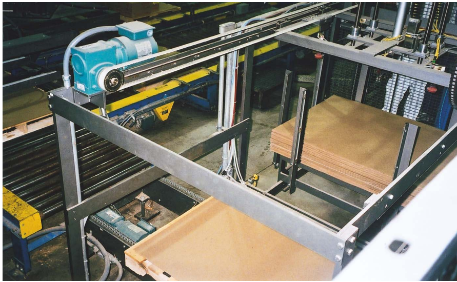
An automatic, built-in basesheet and a pallet dispenser in the workcell are activated, above, to ready a pallet for the case loading/pick-and-place process. Right, one of several aseptic cartoning systems upstream outfits each drink-pack with a flip-cap.
