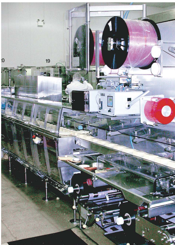
The new easy-open/reclosable package is hermetically sealed on a semi-automatic line that runs 150 200-g packs/min.
