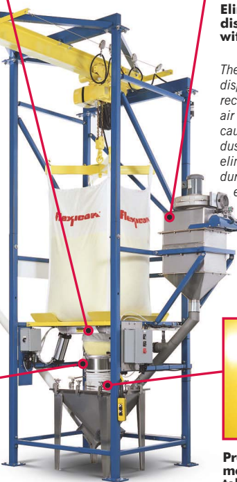
Cinch spouts concentrically with POWER-CINCHER® flow control valve*
