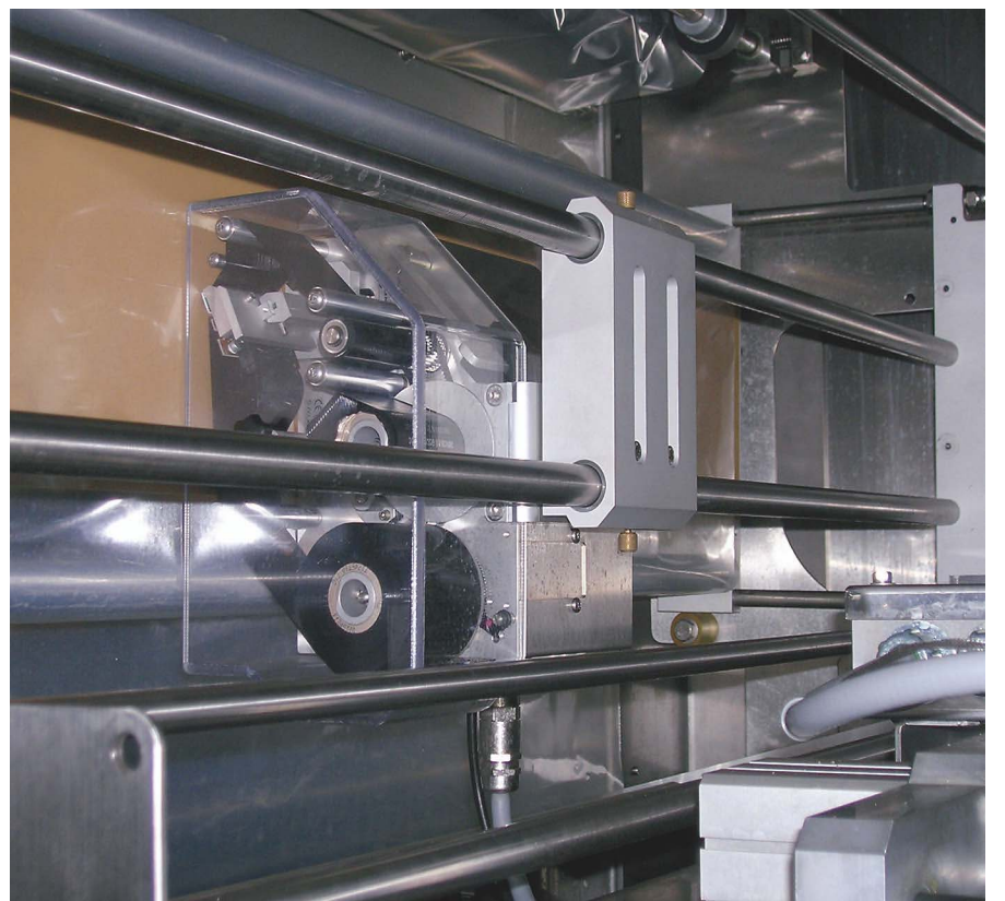
The intermittent TTO uses a 2-in.-wide, black wax/resin ribbon to print a batch number and an expiration date onto clear, PP rollstock before the film is formed, filled with sour cream and sealed in a new vf/f/s machine.
